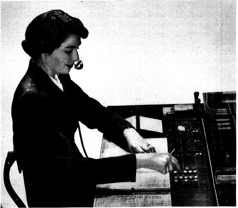
Fig. 12—Toll switchboard position with key set used for toll dialing.
