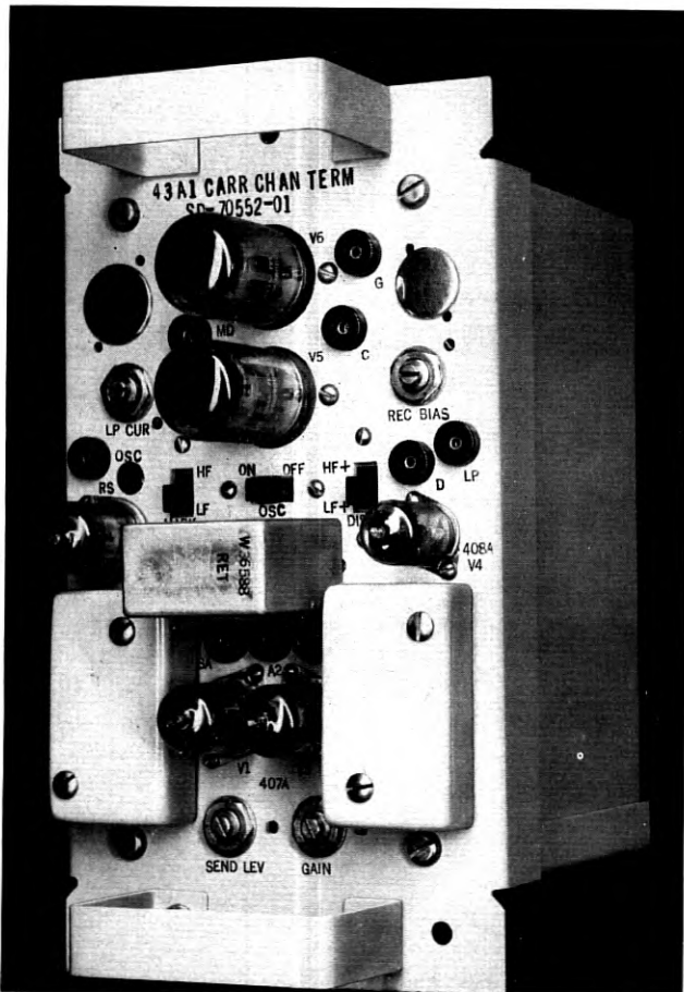
Fig. 7—Channel terminal, front view.
