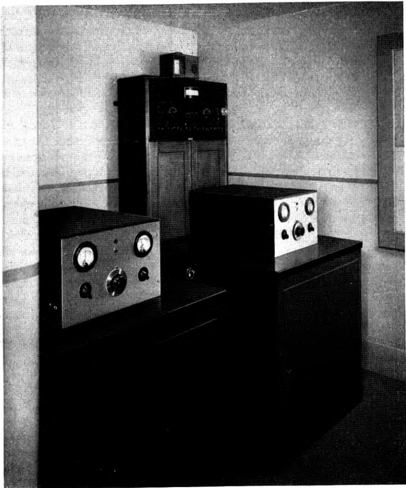
Fig. 29—Two of the four quartz oscillators of the Bell System Frequency Standard, 1937 to date.
