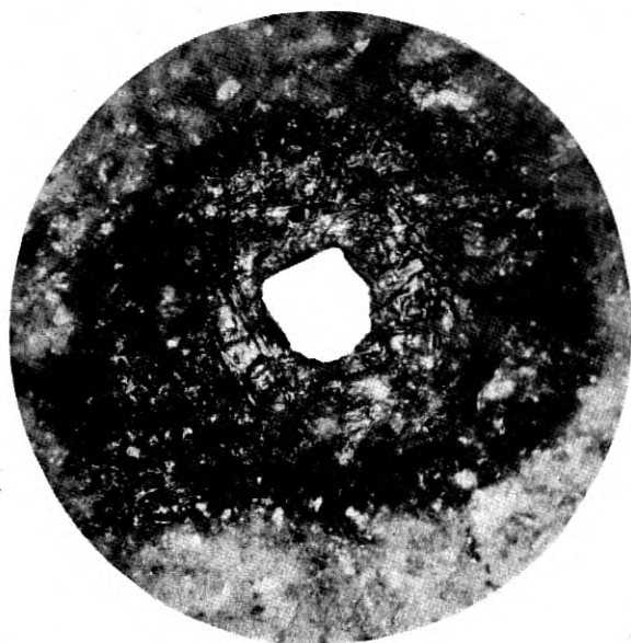
Fig. 28—Photomicrograph of single spark record showing nature of recording on wax-coated chart paper. \times 100
