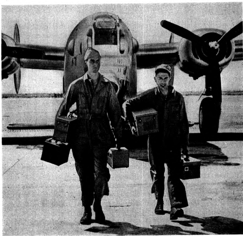
Fig. 3—Portable units used in checking airborne radars at Boca Raton, Fla.
