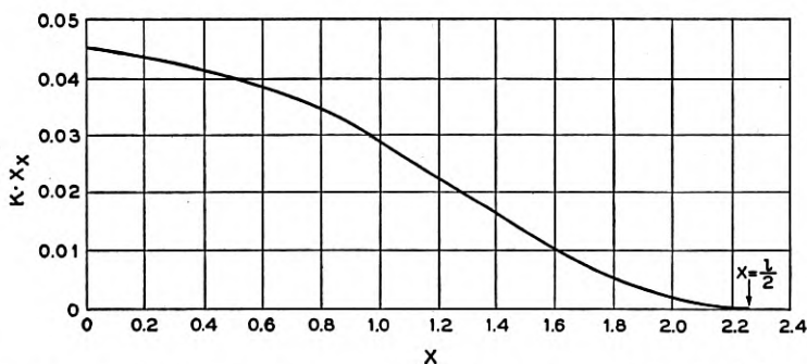
Fig. 7.13—Distribution of longitudinal stress for free-free bar vibrating in first flexure mode
