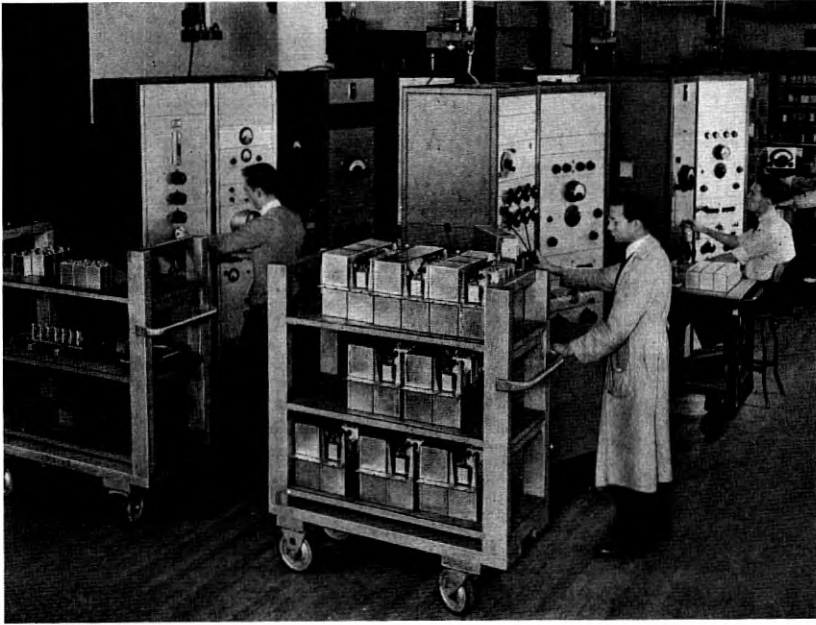
Fig. 12—Filter testing area. The standard-frequency outlets are seen above the test sets.
