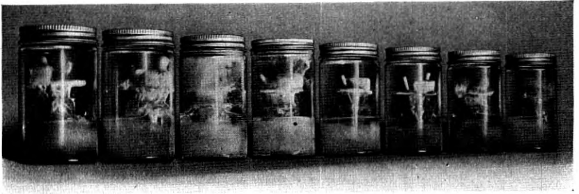
Fig. 10.—Assay of worthless preservative at maximum concentration. The fungi in duplicate from left to right are Lenzites trabea , U-10, Fomes roseus and Lentinus lepideus .
