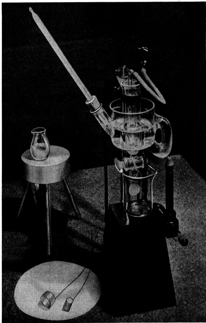
Fig. 4—With this electrolytic cell as little as a milligram of various heavy metals may be precisely determined.
