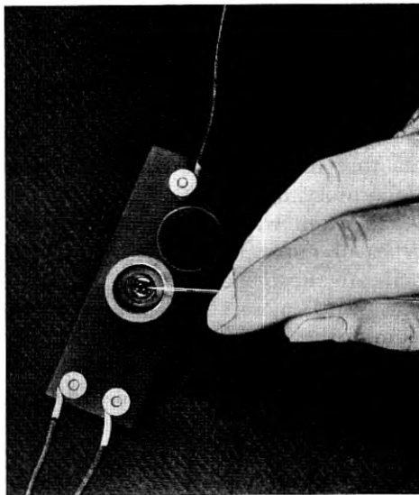
Fig. 3—The electrolysis cell shown here, when used under the microscope, permits one to observe the deposition of metals from tiny drops of solutions. Less than a thousandth of a milligram of copper or zinc may be detected by its use.
