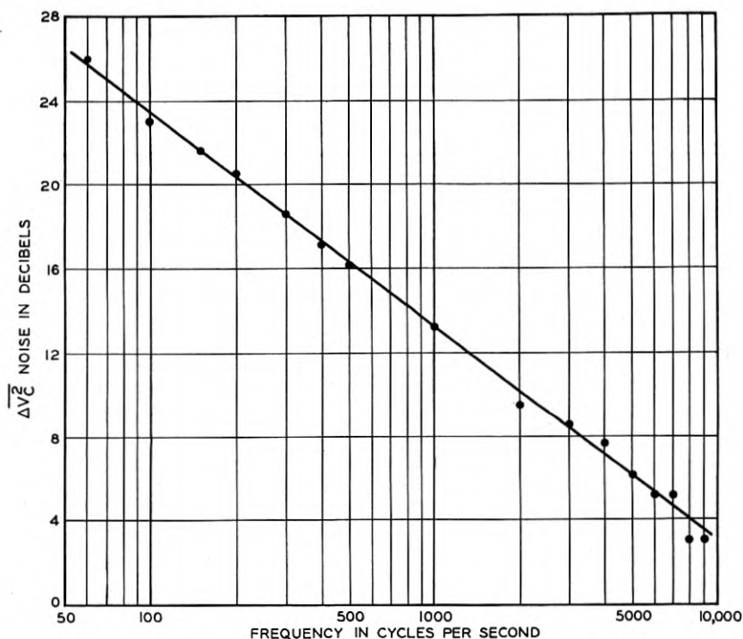
Fig. 10—The frequency distribution of contact noise in a standard carbon transmitter for normal operating conditions. The ordinates give the mean square contact noise voltage in a twenty-cycle band the midpoints of which are given by the abscissæ.
