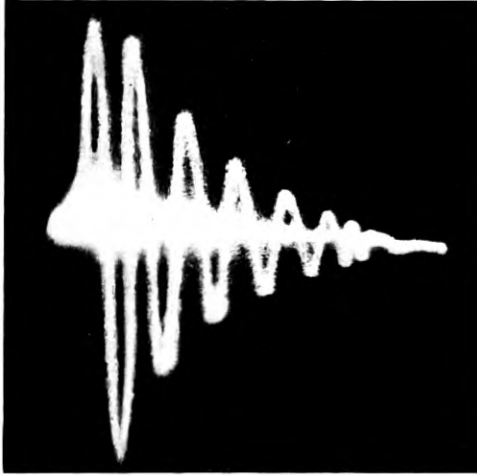
Fig. 23—Discharge of condenser through inductance.
