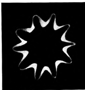
Fig. 34—"Gear wheel" frequency comparison, ratio 10 : 1.
