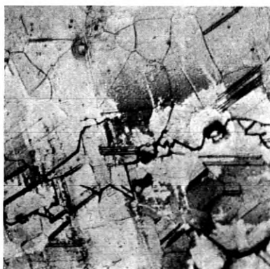
Fig. 11—Photomicrographs of Fatigue Specimens.
