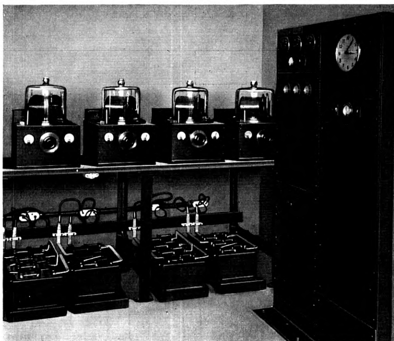
Fig. 17—Four 100,000-cycle oscillators with auxiliary equipment.
