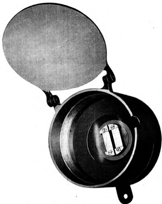
Fig. 6—Thermophone in chamber for calibrating transmitter.
