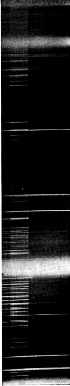
Fig. 4—Light scattered by benzene (with comparison spectrum). The four fat lines from left to right are 4046, 4358, 5461 and the doublet 5770-5790 of the unshifted scattered light. (R. W. Wood.)
