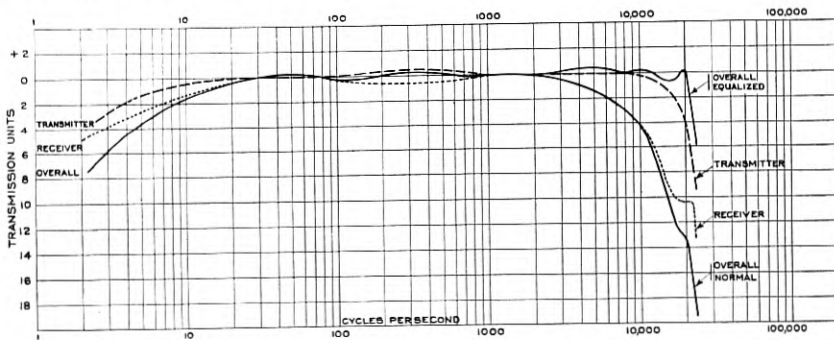
Fig. 7—Measured characteristics of television channel
