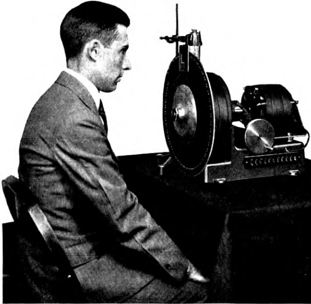
Fig. 6—Illustrative receiving apparatus. A neon lamp operated from the picture current illuminates a series of small apertures as they pass across the field of view; the observer sees an image reproduced in the frame.
