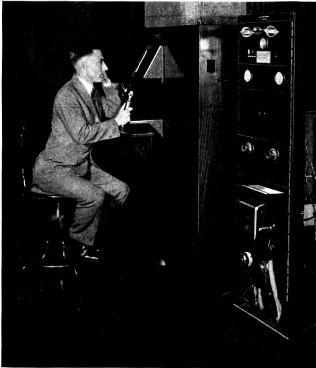
Fig. 8—Disk receiving apparatus. The observer looks through the shielding window at a picture on the 36-inch disk
