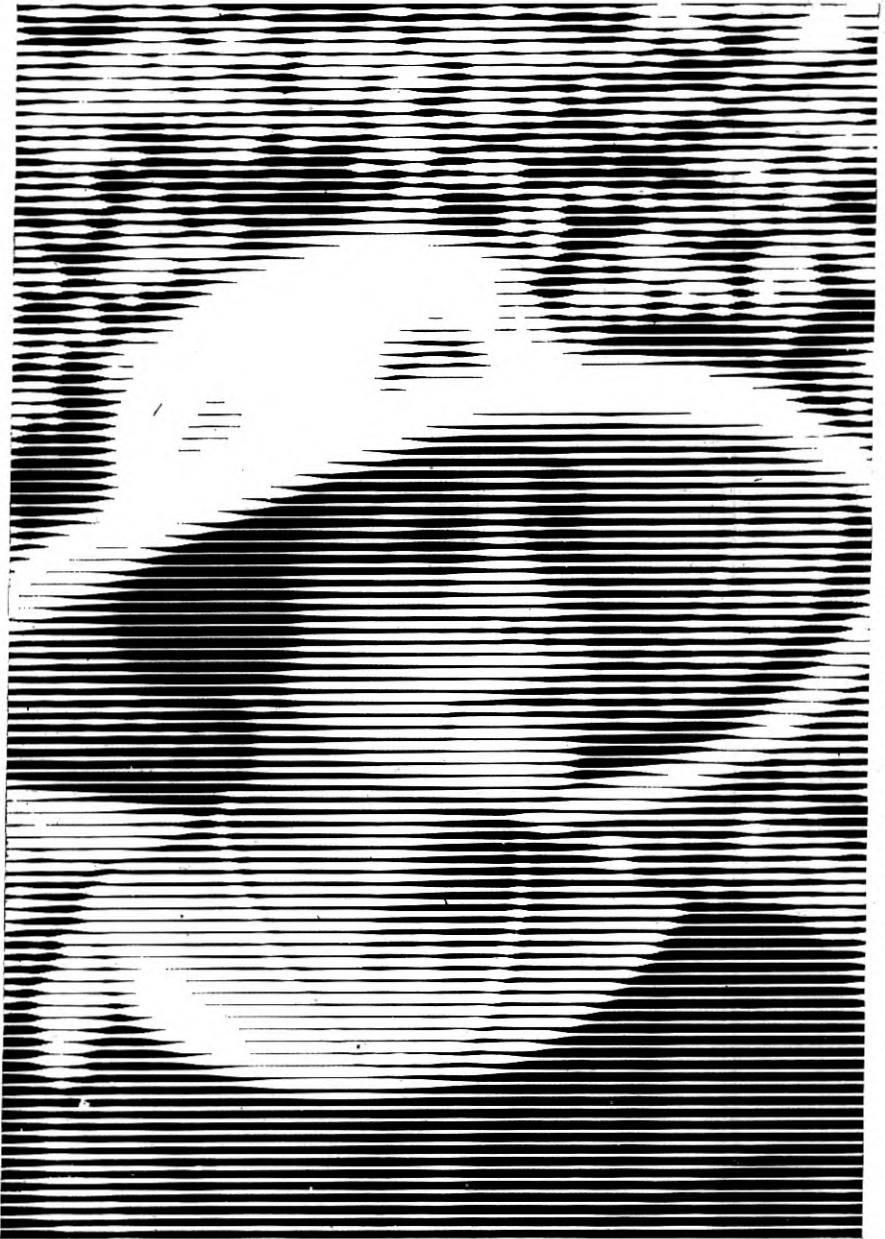
Fig. 5—Portion of transmitted picture of variable width line type, enlarged
