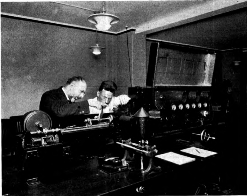
Fig. 7—Sending end apparatus showing motor, film carriage, optical system and amplifier modulator
