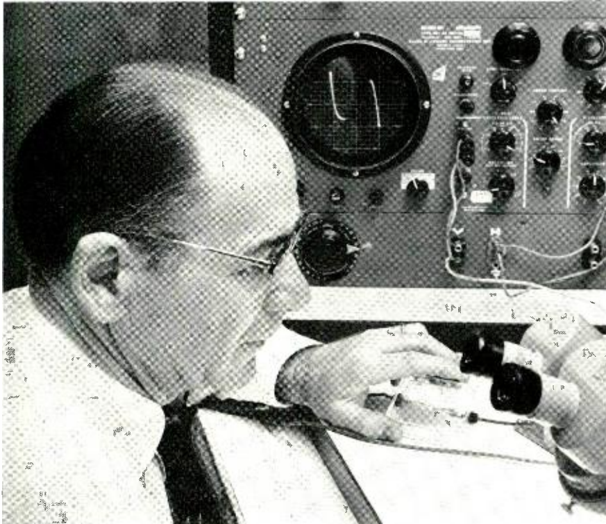
E. Dickten operates equipment that adjusts alloy of Esaki diode by current pulse through device. Oscilloscope picture of voltage-current characteristic indicates type of junction acquired.
