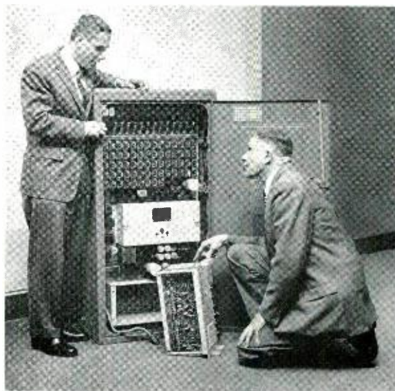
George Parker, left, and Eric Graber with station-control cabinet. Cabinet houses the relay-control circuit and the electronic director.
