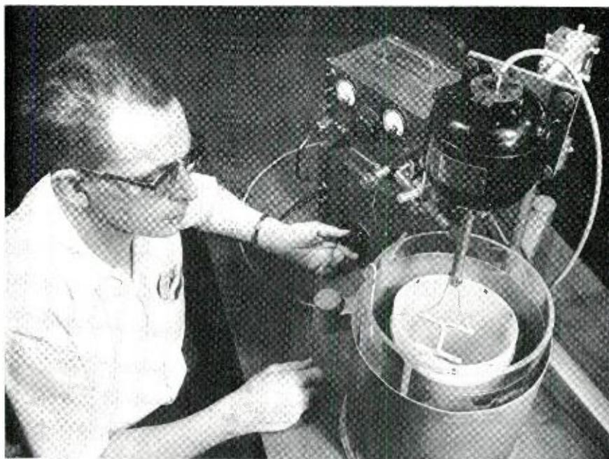
N. J. Pierce adjusts agitating equipment used in electroforming process. Mandrel is slowly rotated in plating bath, first in one direction, then in other. Polyethylene cylinder between tank and part acts as shield to lengthen path.
