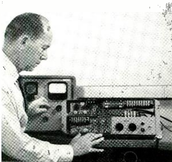
Components of new program amplifier are assembled on recessed chassis, arranged for mounting on 19-inch relay rack or cabinet. Amplifier takes up 7 inches of vertical rack space, is 8½ inches deep, projects 7 inches behind mounting surface.
