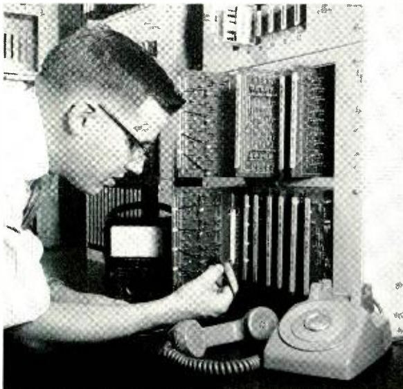
High-speed solid-state devices make possible time-division switching. Printed-circuit boards, shown here being tested, make up most of ESSEX units.
