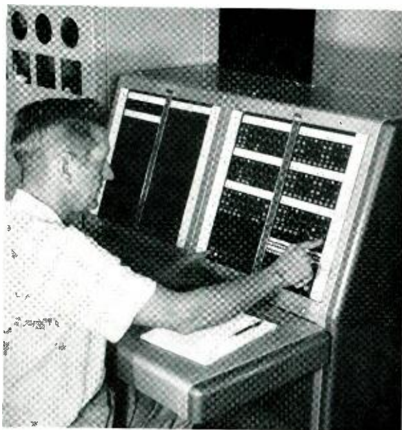
Control console for a typical main station. Operator is demonstrating how "master operate" key and an individual order button must both be pressed to send an order. Keys and lamps for "roll call" are located at the bottom.
