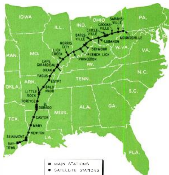
Map showing the route of the Little Big Inch Pipeline. Squares are main stations of SC2 System, as it was originally conceived, and circles are satellites. The direction of flow is north.
