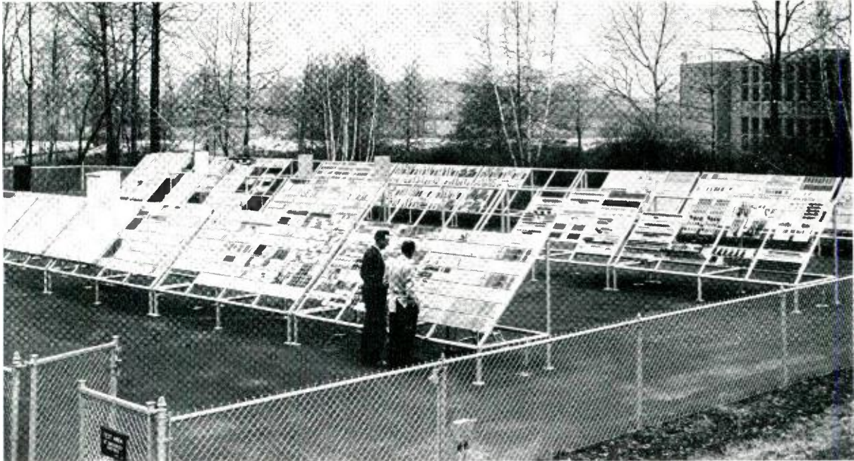
Exposure plot at the Laboratories Murray Hill location. This area is used to weather-test all
