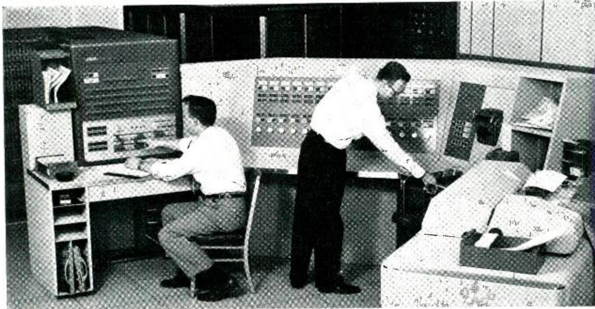
A large proportion of simulation of engineering projects is carried out on this IBM 704 digital
