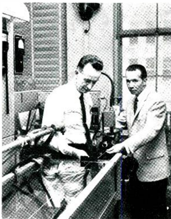
J. B. Howard and V. T. Wallder examine operation of extruding machine. Wire from rear passes through device to receive its “coat” of insulation. It then goes into cooling trough, foreground.
