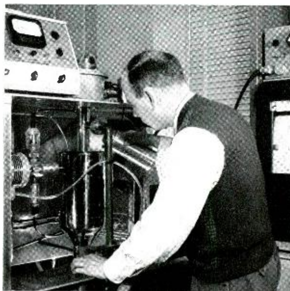
Hall-effect apparatus. R. A. Logan adds liquid nitrogen to super-cool sample in an experiment for measuring the properties of semiconductors.
