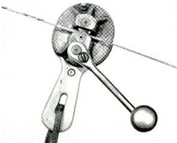
Standard Bell System rolling tool with galvanized steel sleeve and wire held between the rollers.
