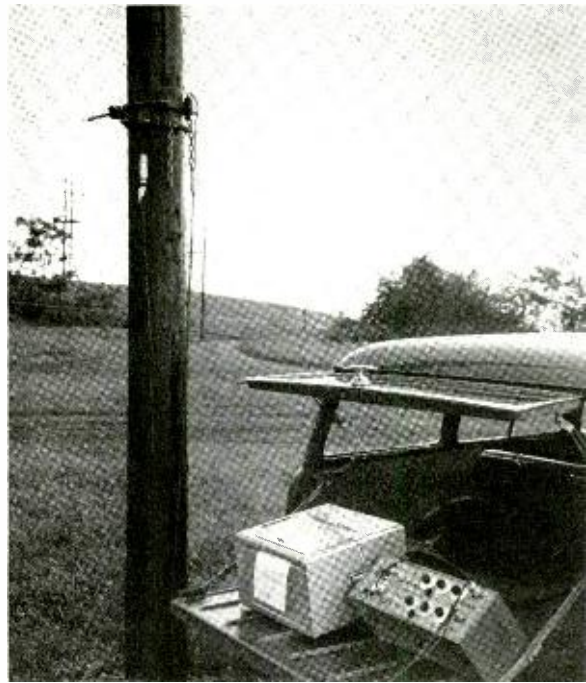
Signals from pole-mounted magnetic pick-ups furnish data for "in the field" vibration studies.
