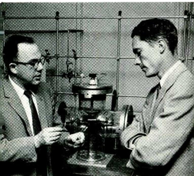
H. Basseches, left, and R. W. Berry examine an experimental circuit sputtered onto a standard glass microscope slide. The T-shaped glass apparatus in background is the evacuated sputtering chamber.
