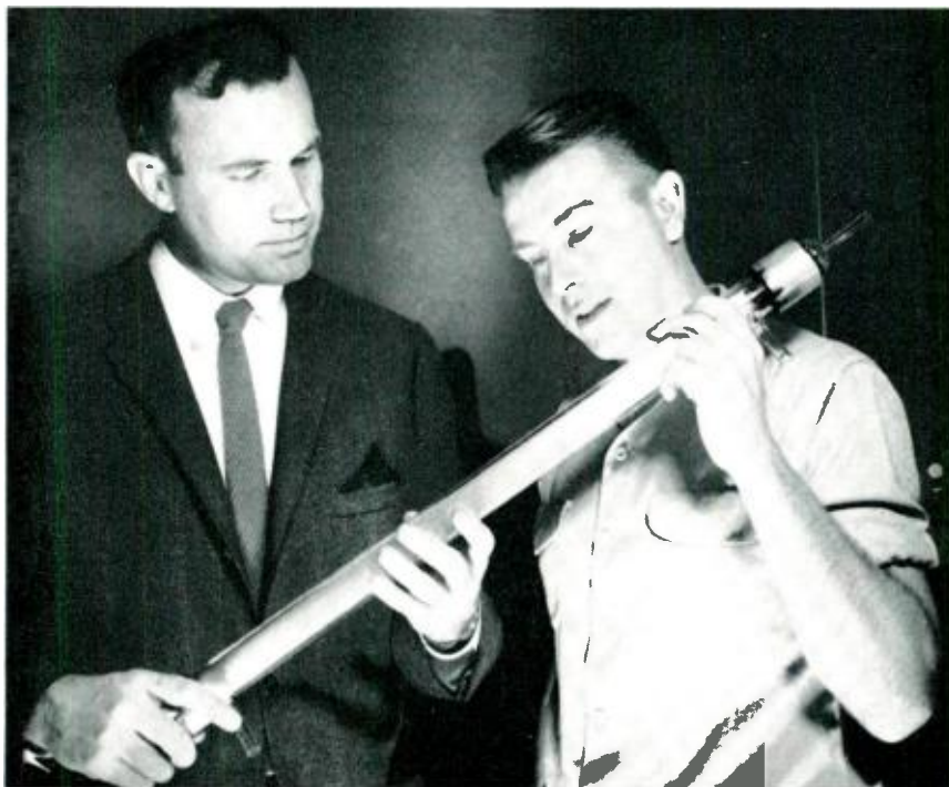
K. B. McAfee and H. Kraft examining experimental cell built to study separation of helium from gaseous mixtures. Gas mixture circulates
