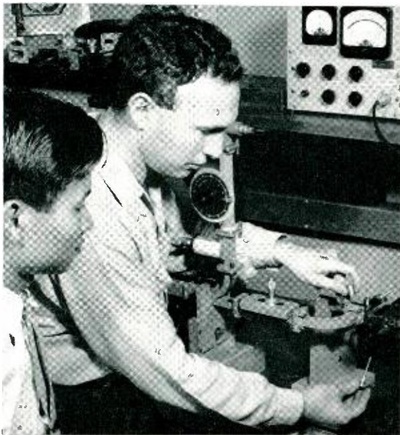
M. Uenohara, left, and G. F. Herrmann prepare to insert new semiconductor diode into equipment for studying diode's amplifying properties.
