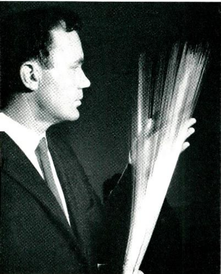
K. B. McAfee holding a bundle of capillary tubes of the type used for helium diffusion. These tubes have an outside diameter of 0.015 inch and a wall thickness of about 0.003 inch.
