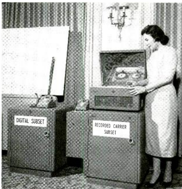
Left: a Digital Subset for immediate transmission of data; and right: a Recorded Carrier Subset which stores many types of data on magnetic tape.
