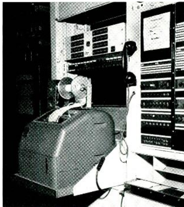
Fig. 3—Registers which score number of deviations in various decibel-bands, seen above teletypewriter which records results of tests.
