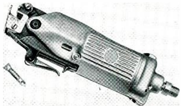
Fig. 1 — Pneumatic presser and sleeve used in punched-sleeve cable splicing. The sleeve assembly consists of a tube made of the same metal as the conductors to be joined (aluminum or copper) with a jacket of plastic that is closed at one end.
