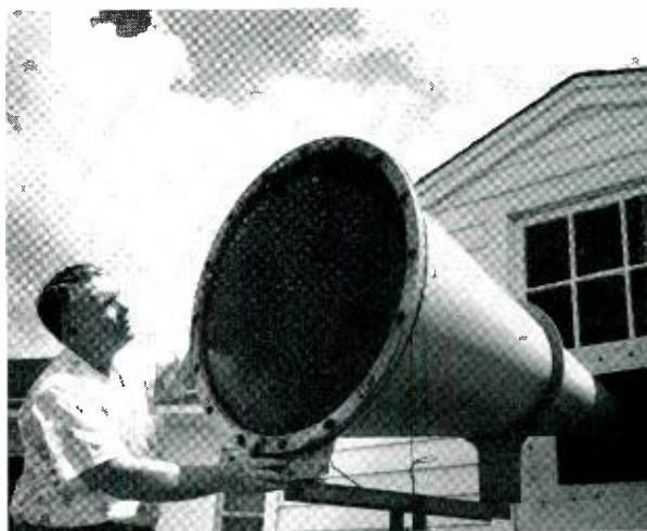
Fig. 2— R. A. Desmond inspecting polyethylene lens on conical horn antenna. Antenna served for both transmitting and receiving the test signals.
