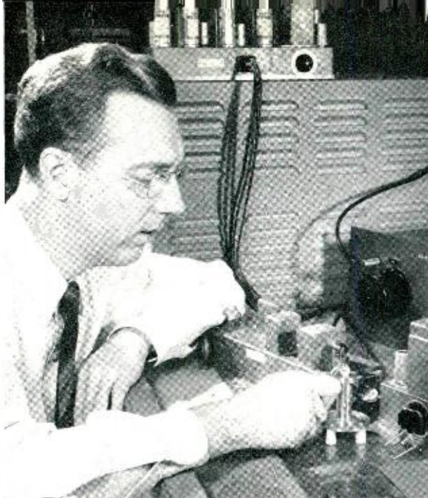
H. J. McSkimin adjusts diamond specimen on the end of fused-silica "buffer" rod.
