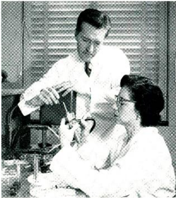
Fig. 3 — Miss M. R. Daly and A. R. Strnad constructing electron gun assembly, a step in the fabrication of the backward-wave 5-mm oscillator tube.
