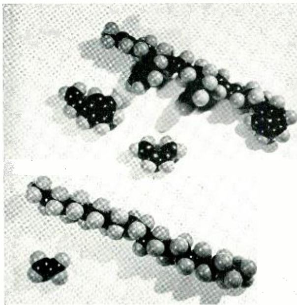
Fig. 1 — Fisher-Hirschfelder-Taylor models of: (from the top) butadiene-styrene copolymer (GRS); butadiene monomer; styrene monomer; polyethylene polymer; ethylene monomer.
