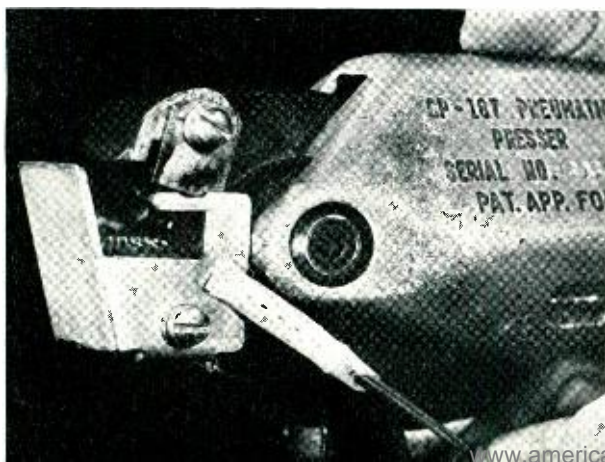
Two conductors after being removed from the presser used in making the punched-sleeve splice.
