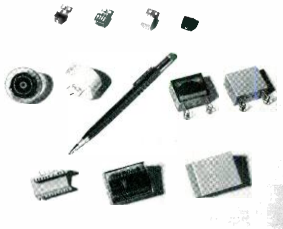
Fig. 5—Samples of miniaturized components showing how polymer materials are used for potting. Units in clear resin were made to show details of inside construction.
