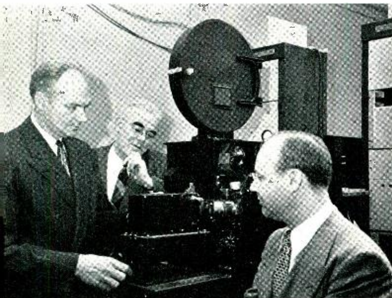
Motion picture film is frequently used as a source of picture signals for transmission studies. This continuous film scanner, developed in the Laboratories, provides signals of sufficiently high quality for advanced visual research. Left, to right, C. F. Matke, A. G. Jensen and R. E. Graham.
