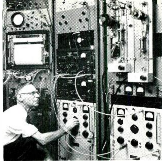
Fig. 7 — W. A. Yager adjusting the automatic frequency control of equipment used for ferromagnetic resonance experiments.
