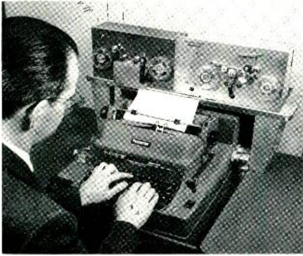
Fig. 3—The author with automatic electric typewriter and experimental equipment for use of magnetic tapes to store data for transmission.
