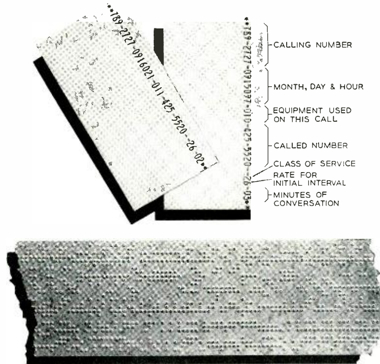
Fig. 2 — Comparison of two printed tickets with a perforated AMA tape carrying the information listed on the ticket for many more calls.
