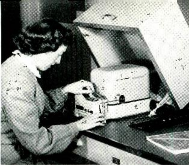
Fig. 4—Punched instruction tape being loaded into an input station of the Model VI Computer by Ann Madden.
