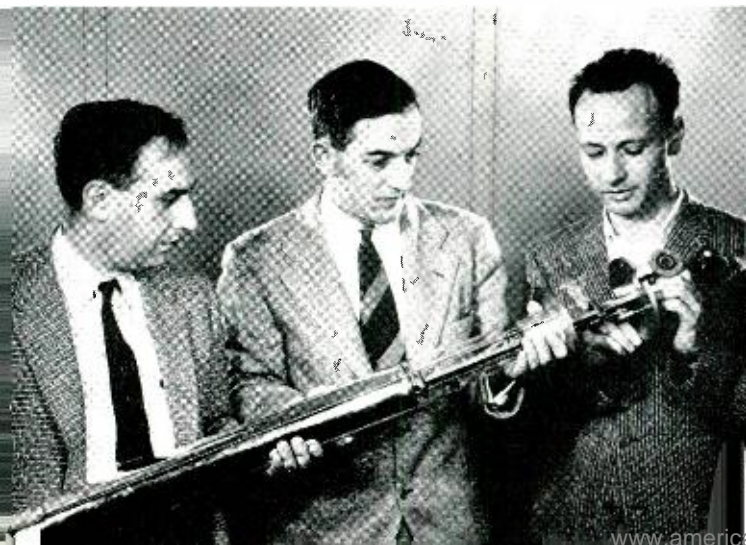
Harold Seidel, Derrick Scovil and George Feher, left to right, with microwave apparatus used to test the solid state devices in a strong magnetic field.
