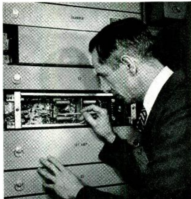
Fig. 3 — R. W. Clausen, New York Telephone Company, inspecting amplifier circuit of A2A equipment used in New York City field trial.
