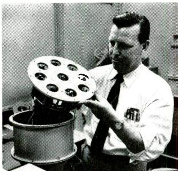
Fig. 4 — W. L. Bacom installs turret in dust meter.
