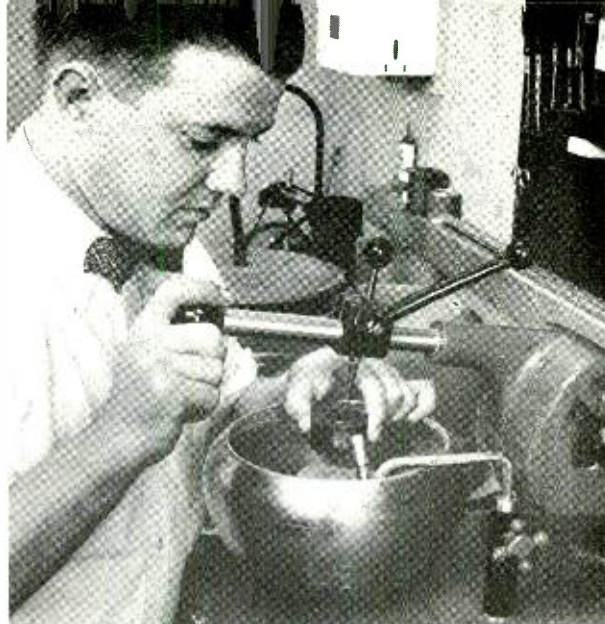
Fig. 7 — E. Berry placing crystal holder in polishing machine prior to beveling operation.
