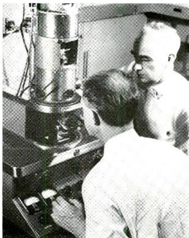
C. J. Calbick, left, and S. M. Arnold get a closeup view of the make-up of some metal whiskers through an electron microscope.
