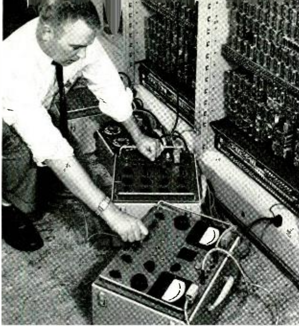
Fig. 1 — W. R. Rupp calibrates the 3A pulse generator. The 3A digit-control set is just back of the pulse generator. The power supply unit is located in the fourth box at the rear of the test-set group.
