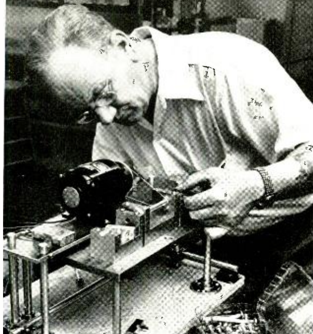
Fig. 6.—J. W. Bell assembling a 5 mm phase-shifter for use in a microwave measuring set.
