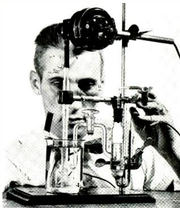
Fig. 6—W. W. Bradley of the Chemical Research Department performing electrode potential experiment as part of laboratory study of corrosion.
