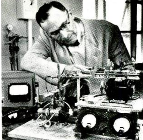
Fig. 5 — A. P. King adjusting a 5 mm single-oscillator, double-detection measuring set.
