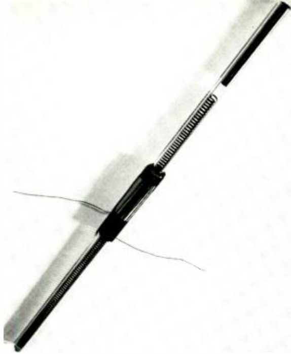
Fig. 6 — Cylindrical ferrite over tube helix as used in the original attenuation experiments.
