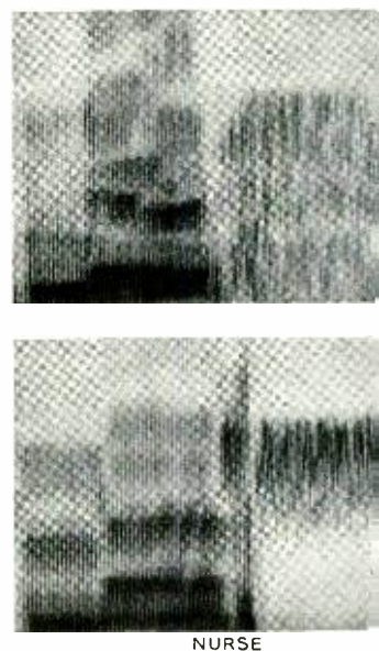
Fig. 6 — A comparison of visible speech spectrograms of the word "nurse" as spoken directly (shown above) and as recreated by Audrey (below) shows only small differences.
