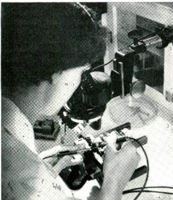
Fig. 7 — Mrs. Betty Haas placing wire attachments on point contact transistor under microscope.
