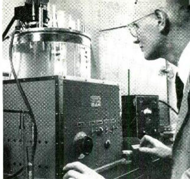
Fig. 7 — W. C. Jordan uses oil bath to determine the viscosity of a polymer solution.
