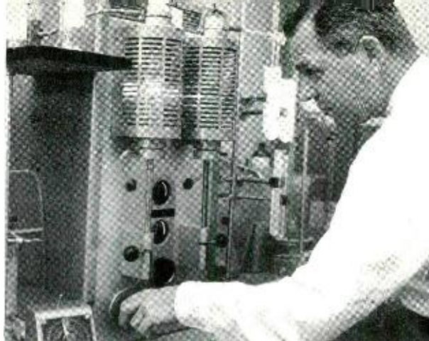
Fig. 4—F. W. Ryan operating the high-temperature induction furnace for carbon determination. The carbon dioxide evolved is collected in the absorption bulb shown in the upper-left corner.
