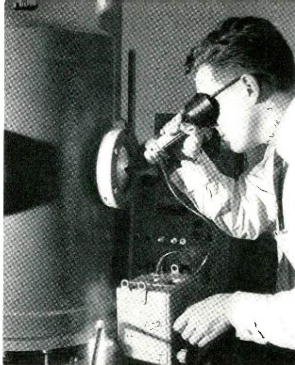
C. A. Lee adjusts optical pyrometer to determine temperature in diffusion chamber where germanium diffused base transistor is made.
