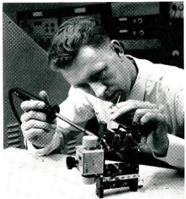
Fig. 4—R. Dempster makes wiring changes on an equalizer network unit.
