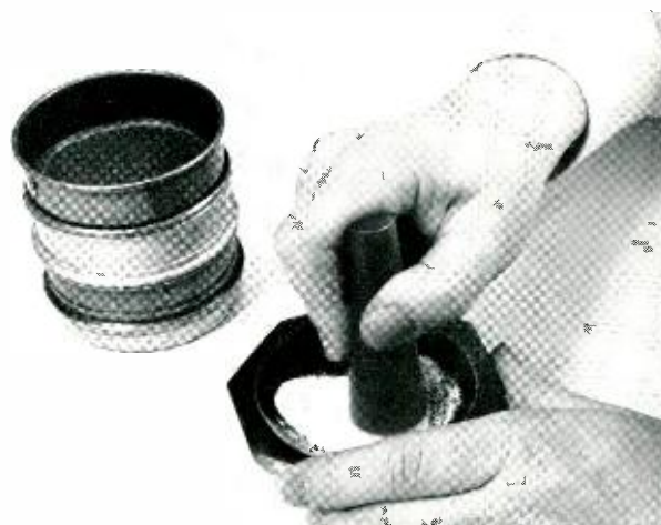
Fig. 7 — Grinding sample prior to use; at left are sieves used to select correct particle size of material.
