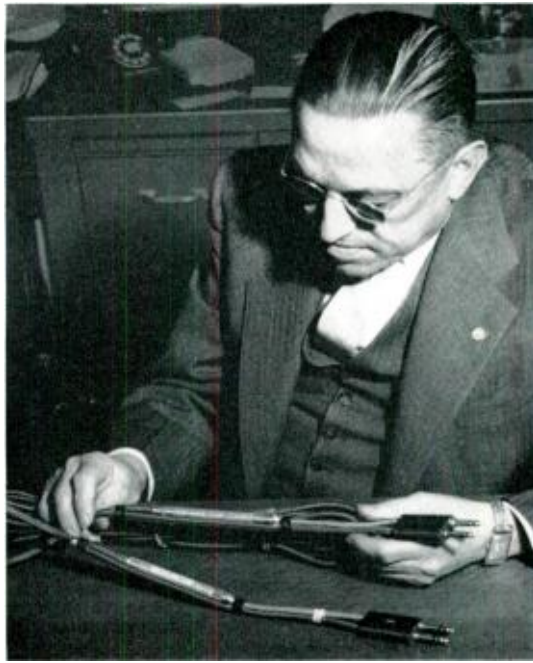
Fig. 4 (left to right) — A. J. Uminowicz inspects a splice that is used in the L3 carrier terminal equipment, A. J. Weir examines an attenuator pad in a channel bank patching cord, and F. W. Koller illustrates the method of installing a pad, using a hand operated crimping tool.
