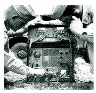
Four-channel cable terminal, AN/TCC-3,
