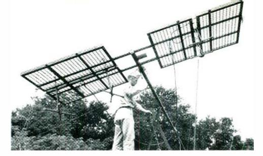
Lowering AN/TRC-24 antennas: gin-pole and block-and-tackle gear permit quick raising and lowering of entire assembly.
