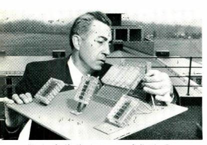
Fig. 1 — D. M. Chapin inspecting Bell Solar Batteries exposed to sun for long term storage battery charging tests.
