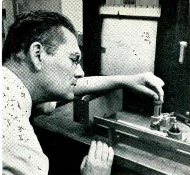
Fig. 5 — J. J. Gillich measuring electrical resistivity along the length of a zone-refined germanium ingot, using an apparatus which automatically brings 4 electrodes down on the ingot at 0.1 inch intervals as it traverses the ingot.
