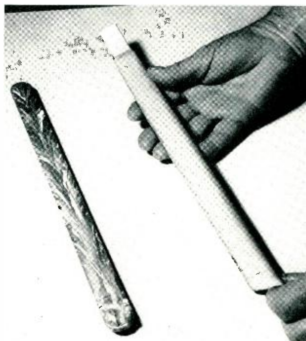
Fig. 7 — A polycrystalline zone-refined ingot of germanium at the left, exhibiting grain boundaries, compared to a highly perfect and highly uniform single crystal zone-levelled ingot.
