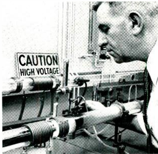
Fig. 4—C. F. Larkin operating the zone-leveling apparatus. In this operation a desired addition agent (antimony) is placed in a single molten zone, which then traverses the ingot, producing a large single crystal of a uniform antimony concentration.
