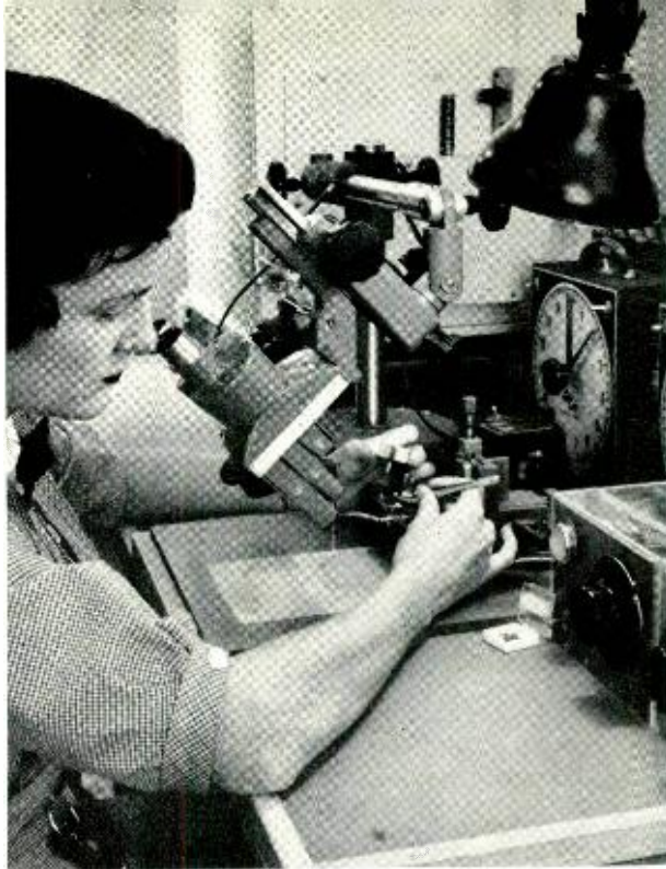
Fig. 8 — Mrs. P. A. Queripel preparing automatic equipment for alloying p and n wires in the fabrication of silicon alloy semiconductor diode.
