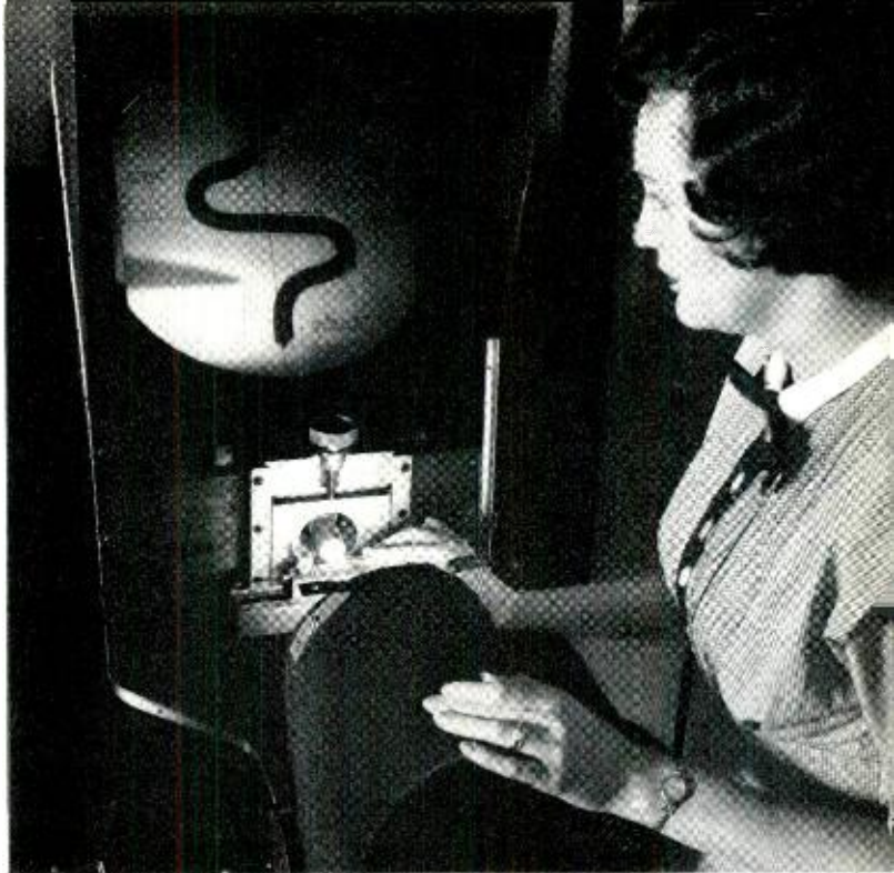
Fig. 5—Mrs. P. A. Queripel inspecting enlarged image of an "S"-shaped spring used in point-contact diodes. Point is later pressed against semi-conductor wafer.
