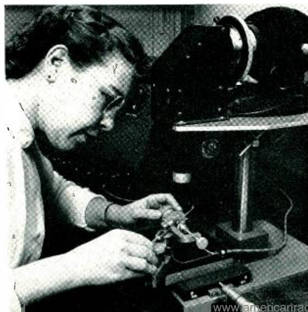
Fig. 6 — Miss L. C. Lovell measuring carrier lifetime of a sample cut from a zone-levelled germanium single-crystal. Such measurements indicate purity, crystalline perfection, and suitability of the germanium for transistor use.
