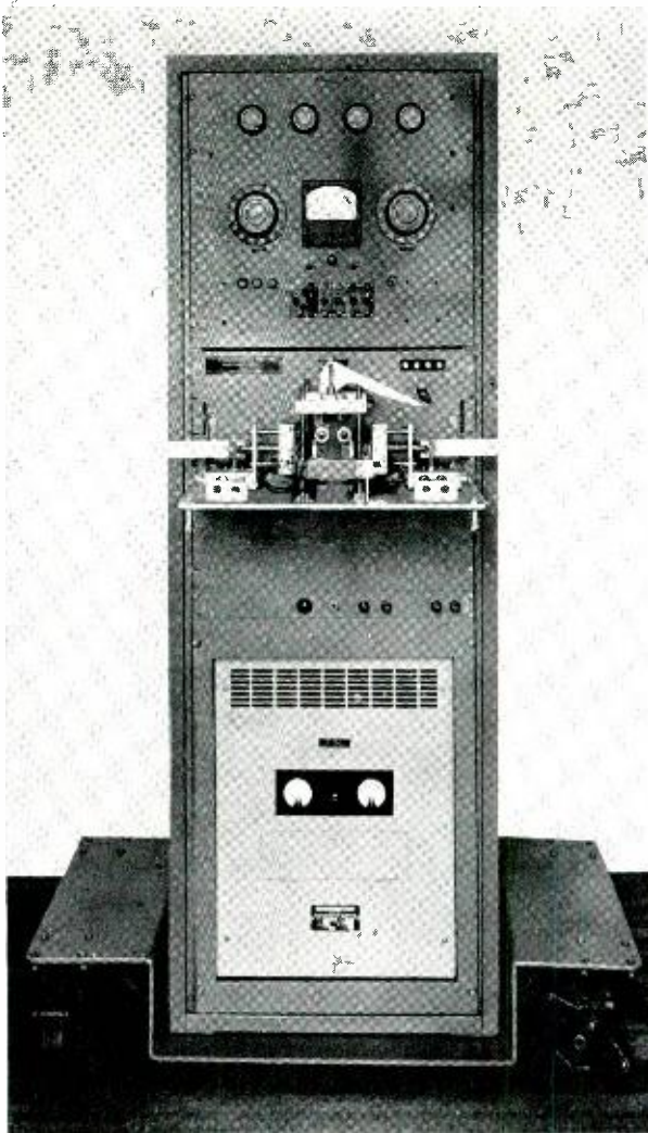
Fig. 4—Western Electric Company equipment for adjusting 223-type switch.
