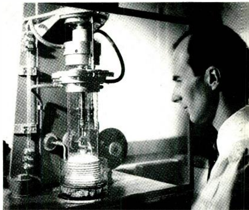
Fig. 3 — E. D. Kolb operating a machine used to grow single-crystal germanium.
