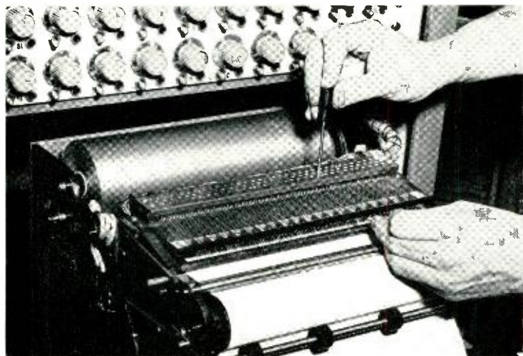
Fig. 3—Set-screws in the pen-carriage assembly permit adjusting the pens individually.
