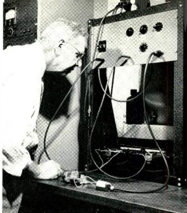
Fig. 5 — R. T. Jenkins checking the performance of a telephone ringer.
