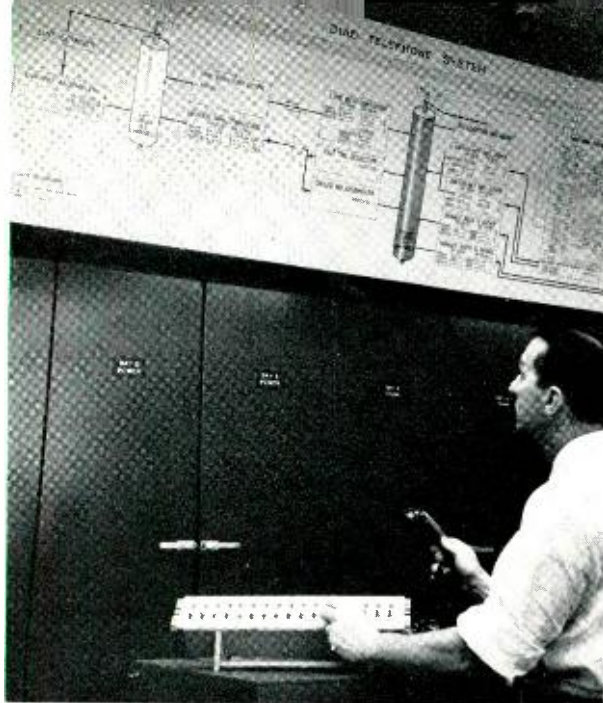
Fig. 4—J. F. Muller placing call at control panel. Display board overhead shows progress of call.
