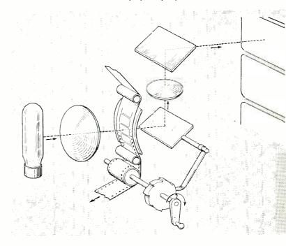
longer be able to fill the projection lens, and will begin to lose light. In other words, we simply run out of mirror area. Theoretically, we could avoid this trouble by allowing the mirror to track the film while it moves through one frame height, then snap it back instantaneously to catch the next frame, and so on.
