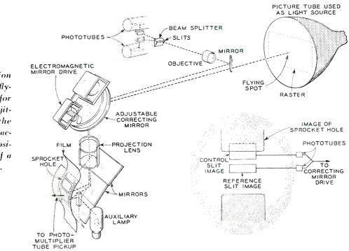
Fig. 4—Combination of projector and flying-spot scanner for televising film. A "jitter" servo adjusts the correcting mirror according to the position of an image of a film sprocket hole.
