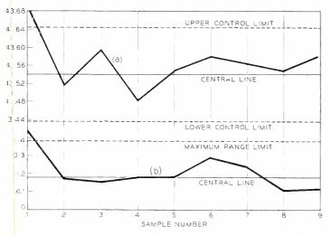
Fig. 3 — Control chart; (a) average of samples of five units each, (b) range of units in each sample. The ordinate scale on this diagram may be considered as being in arbitrary units.
