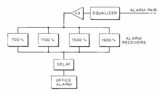
Fig. 4—Block diagram illustrating a typical receiving station.
