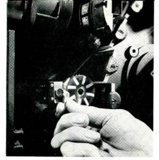
Fig. 5 - A close-up of the film gate and driving sprocket. The relative angles of the mirrors on the drum may be clearly seen.
