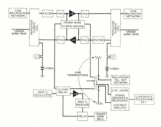
Fig. 2—Block diagram of order wire intermediate repeater.
