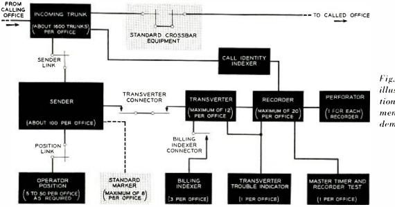
Fig. 1 — Block diagn illustrating the op tion of CAMA equ ment in a crossbar dem office.
