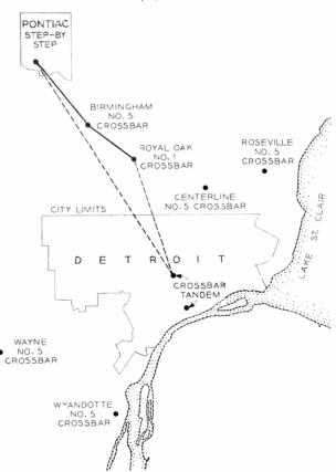
Fig. 1 — Map illustrating use of the No. 5 crossbar tandem revertive-pulse incoming register in the Detroit, Michigan Area. Solid line shows the path of a call from Royal Oak to Pontiac if a No. 5 crossbar office is used and the dashed lines indicate the route that would be required if that office were not available.
