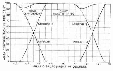
Fig. 6 — The lap-dissolve is not perfect as one mirror slides into the position of another. The slight changes in light efficiency are eliminated by a "flicker" servo.
