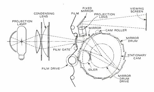
Fig. 2—The simple mirror-and-crank arrangement of Figure 1 has been replaced by several mirrors placed on a moving drum. screen will be just as constant and permanent as though it were painted there. All periodicity of the frame rate will have been completely erased. This means that we can televise this picture off the screen at *any scanning rate whatever* = 30 frames/sec, 2 frames/sec, or 1,000 – it doesn't matter; and, of course, no synchronizing is needed.
