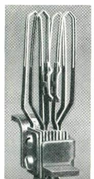
Fig. 3—Nest of eight sequence switch springs. The middle two springs in the' front have been replaced. connected to permit slipping the brush over its upper end. For simpler maintenance, two types of guides have now been provided. These guides, shown in Figure 1, compensate for worn guiding surfaces of commutator brush <sup>f</sup>rames and are easily and quickly attached.
