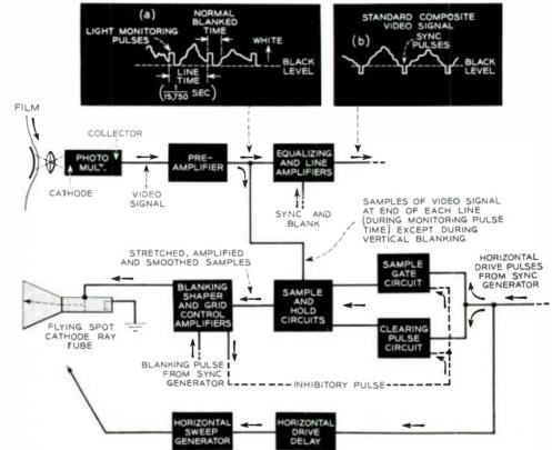
beam intensity is controlled by light-monitoring pulses that have been properly sampled, smoothed, and amplified.
