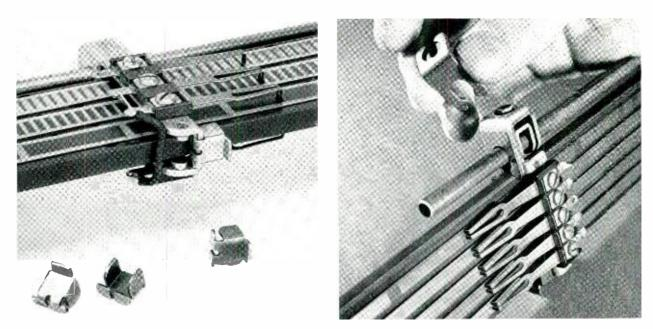
Fig. 1 — The two types of guides supplied for panel system maintenance. The photograph at the top of the page shows author installing a new commutator on a frame in Bell Laboratories panel test equipment.
