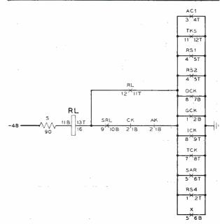
Fig. 2 — A detached contact schematic showing the complete RL relay path. The designations below each contact symbol refer to spring numbers of the top and bottom of each relay.
