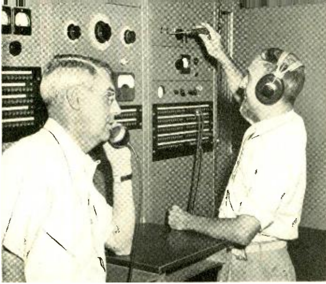
Fig. 1 — R. L. Miller (right) of the Acoustics Research Department and the author at work at the Vocoder. Here vocal sounds are investigated to discover and take advantage of the redundancies of speech as well as to learn more about other speech characteristics.
