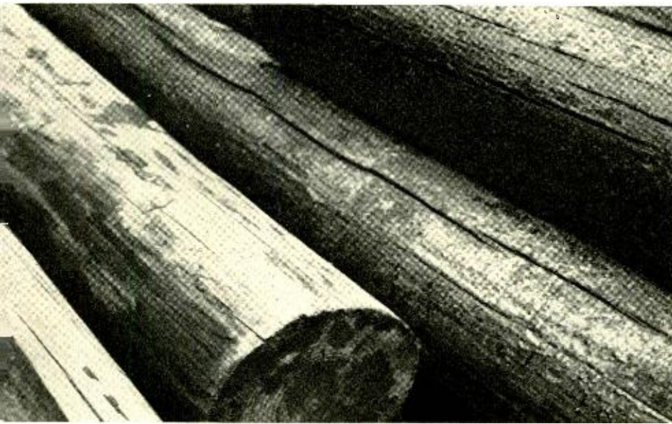
Fig. 1 — Bleeding and non-bleeding telephone poles; bleeders at the right and non-bleeders at the left.
