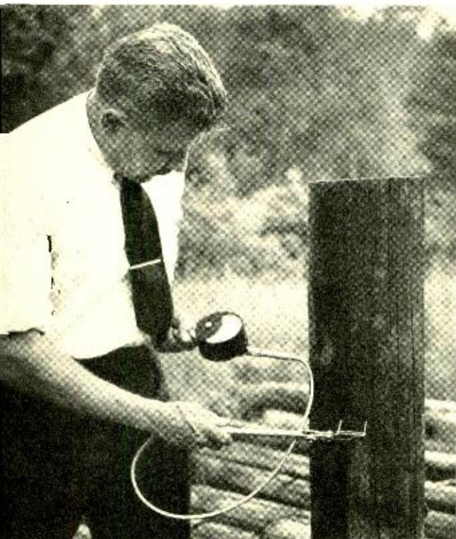
Fig. 3 — A. H. Hearn using a specially developed fine-wire thermocouple to measure the surface temperature of a vertical pole section.
