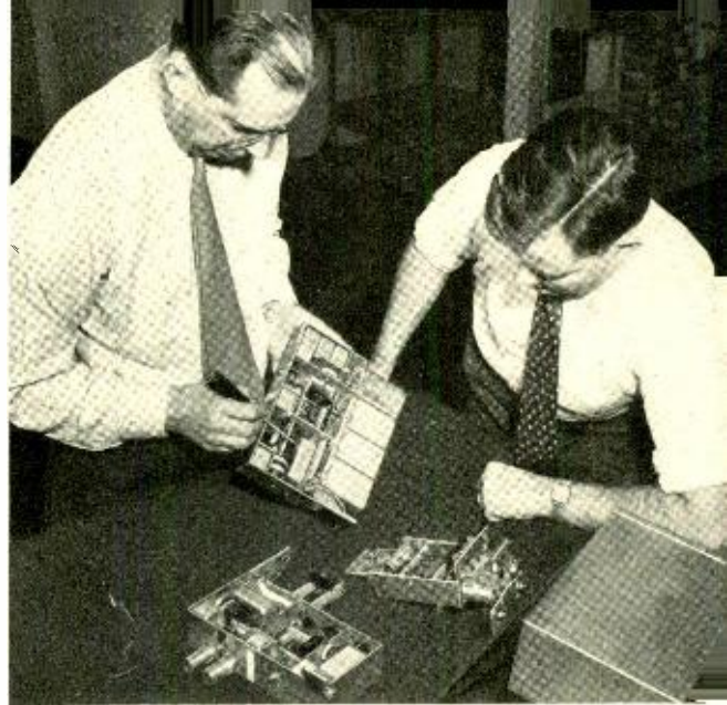
Fig. 1—E. H. Perkins (left) and J. B. Evans are examining the modulator wiring of a laboratory modified repeater.
