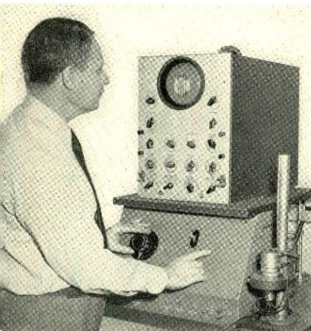
Fig. 6—R. R. Kreisel watches shift in oscilloscope trace as he reduces strength of receiver magnet. Jig for coupling receiver to microphone is seen at right.
