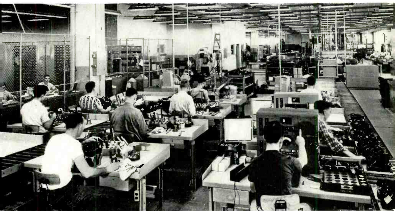
Fig. 1—Portion of a distributing house repair shop—assembly line for hand telephone and telephone set repairs.
