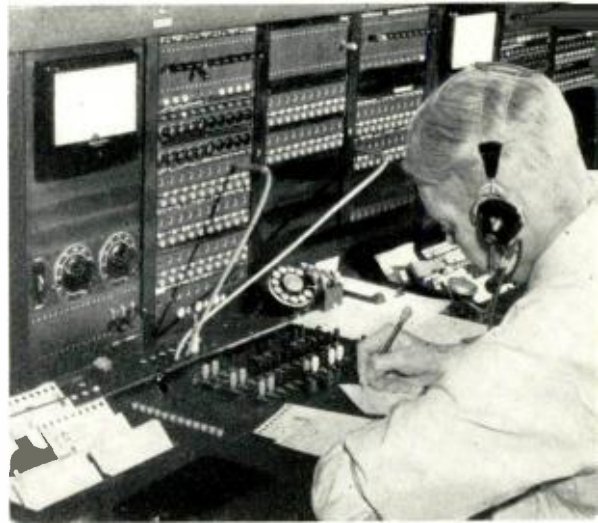
Fig. 4—Close-up of one No. 14 test desk position equipped with an electronic voltmeter and multi-frequency key pulsing. The multifrequency key pulsing set is evident just to the right of the dial.
