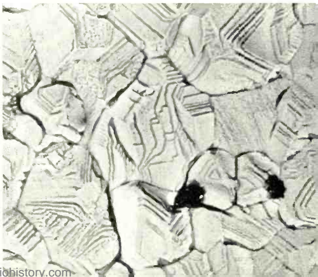
Fig. 6—1150 degrees C—Crystallographic surfaces become pronounced. Magnification 13,000X.
