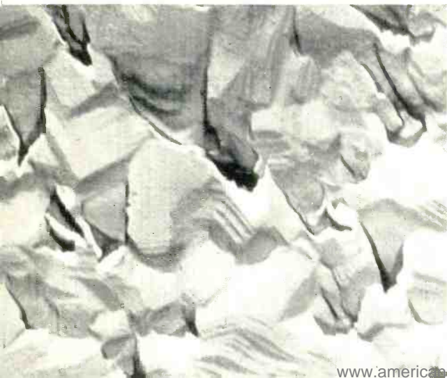
Fig. 5—1100 degrees C—Spaces between particles close, leaving isolated pockets. Magnification 13,000X.
