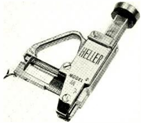
Fig. 2—Hammer-operated stapler permits attachment of JKT wire to plaster.
