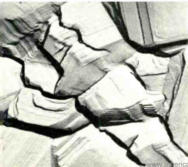
Fig. 9—An alternative treatment uses greatly prolonged heating at 1030 degrees C without the higher temperatures. This produces an extremely compact structure with superior electrical properties. This treatment was developed as a result of electron microscope studies.
