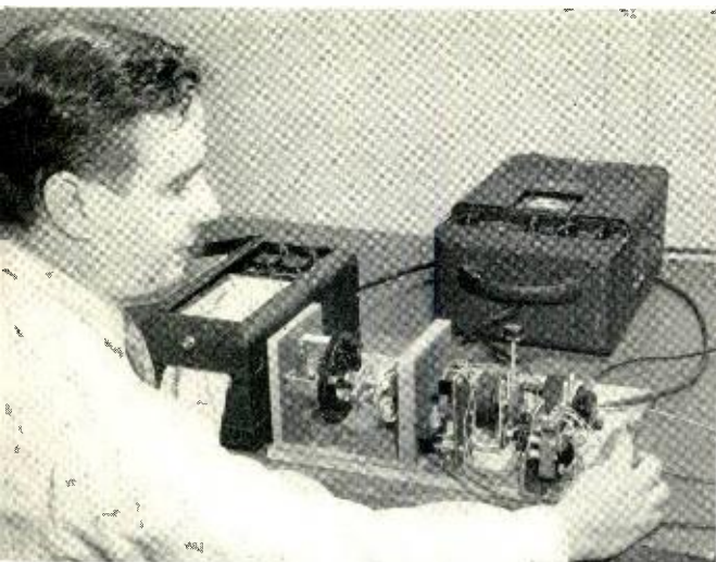
Fig. 5—J. H. Ham determines variations in finger-wheel torque by means of an electromechanical transducer and a recorder.
