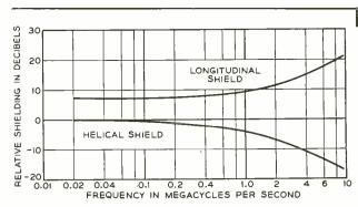
Fig. 2–Improvement in the relative longitudinal shielding gained by using the longitudinal inner shield in the video pair.
