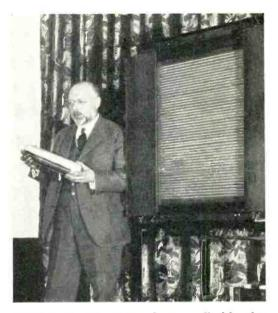
Three of the big photo-electric cells like that held by Dr. Ives were used to convert light to electric signals.
