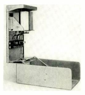
Fig. 2-The 108A protector in its mounting.
