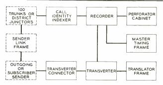
Fig. 1-Seven major equipment units, indicated by solid lines above, comprise the AMA equipment in a central office.
