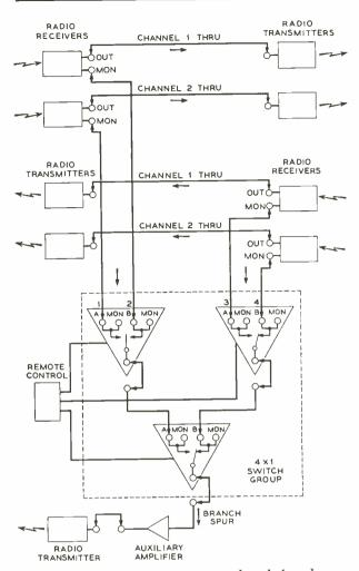
Fig. 10-Typical arrangement employed for dropping off a television channel at an auxiliary repeater station. Patching is set up permanently, but the switching is carried out by remote control.
