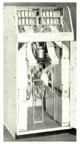
Fig. 2–A perforator cabinet houses two perforators and their tape supplies. Below the perforators on either side are the paper input bins, and between them are the motor-driven reels for storing the output tape from the perforators.
