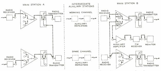
Fig. 5-Method of patching at each end of a defective link to substitute a spare channel.
