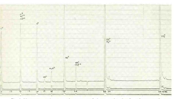
Fig. 3-Mass spectrum of a mixture that is composed of neon, carbon dioxide, carbon monoxide, nitrogen and water.
