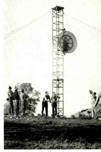
Part of the job of creating a microwave relay route is the survey which tells whether there is a satisfactory line-of-sight transmission path between two proposed station sites. It is made by setting up portable towers developed in the Laboratories (RECORD, January, 1948, page 6) and running a movable antenna and reflector up and down. These pictures were taken by G. M. Eaton of the Pacific Company.
