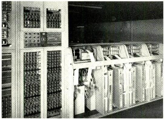
A typical accounting center machine showing relays and miscellaneous equipment in the tall cabinets at the left, a reader in the first low cabinet, and perforators in the other low cabinets.
