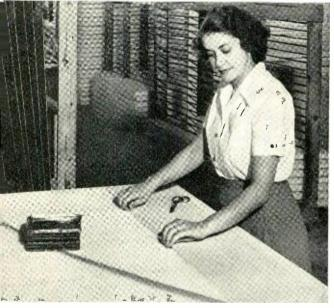
Fig. 3 – Placing the aluminum strips in the slots. 52
