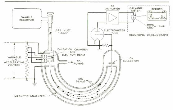
Fig. 2-Schematic diagram indicating the principles of operation of a mass spectrometer.
