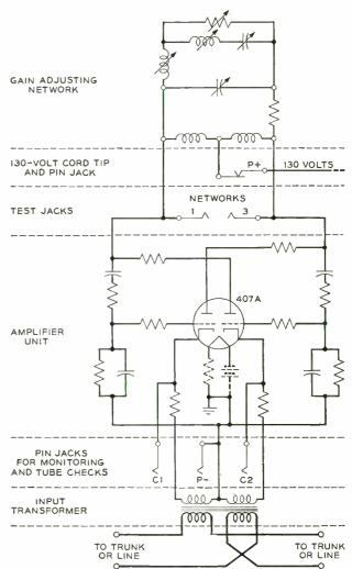
Fig. 4- Simplified schematic of the E1 circuit.
