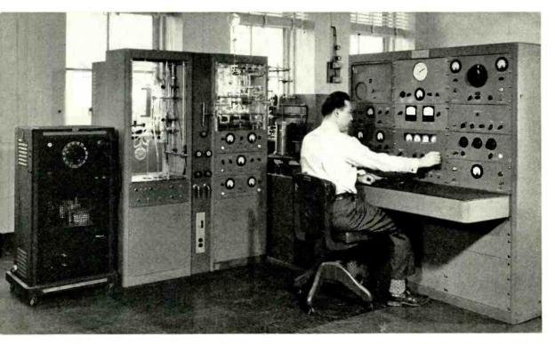
Fig. 1-E. E. Francois operating the mass spectrometer. The instruments shown above and in Figure 4, and the Diatron, were developed by the Consolidated Engineering Corporation.
