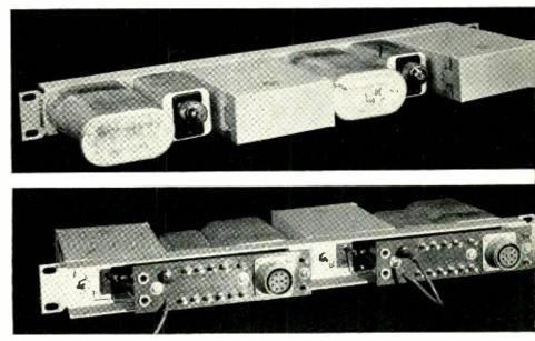
Fig. 1-Two complete repeaters are supplied on a single nineteen-inch plate: front view at the top, and rear view at the bottom. Each repeater, as shown from left to right on the front consists of an input transformer, an amplifier unit, and a gain - adjusting network.
