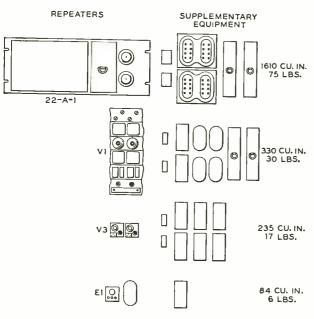
Fig. 2-Size of the E1 repeater compared to that of other types.
