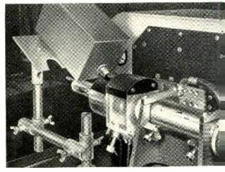
Fig. 3–Viewing unit in place for controlling a braze on a copper tube.
