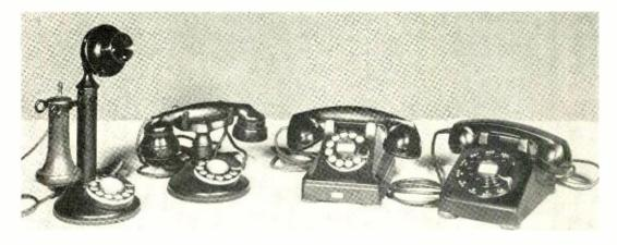
Fig. 1-Left to right, the deskstand of 1919, the handset of 1927, the combined set of 1937, and the 500-type set of 1950.
