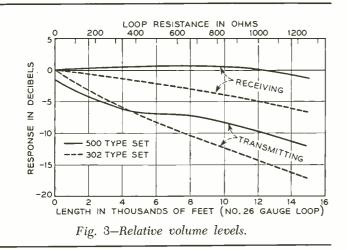
the filament resistance is negligible. Because of the negative coefficient of resistance of the thermistor a corresponding graduated receiving loss with change in loop is obtained. Thus, the higher gains of the new transmitter and receiver are permitted to work to full advantage on long loops but are reduced on short loops to keep the over-all level approximately equal to that of the 302 set.
