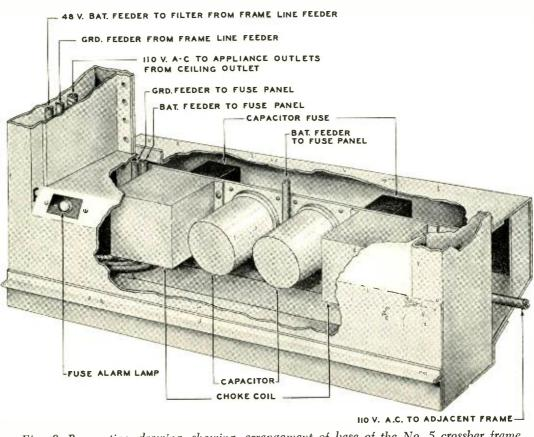
Fig. 6-Perspective drawing showing arrangement of base of the No. 5 crossbar frame.
