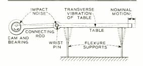
Fig. 3–Reciprocating vibration testing machine with table supported by flexure plates.
