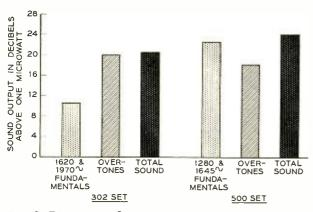
Fig. 6-Ringer sound output spectrum.
