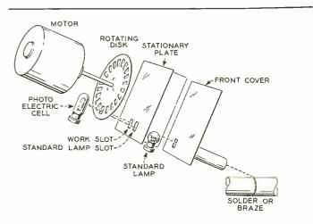
Fig. 1–Optical commutator for temperature control.
