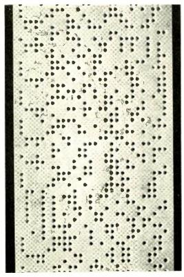
Fig. 1–A section of AMA tape after it has been perforated.
