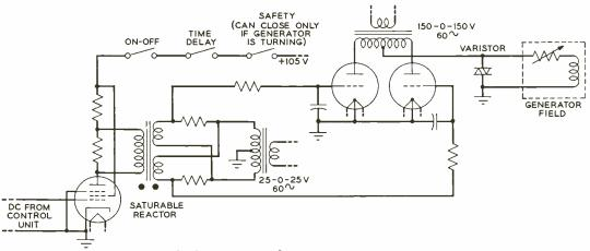
Fig. 7-Schematic circuit of field current supply.
