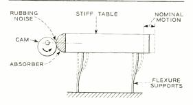
Fig. 4-Schematic arrangement of new leaf spring machine.
