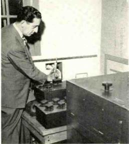
Above right, G. I. Schaible is making connections to a cable under test preparatory to measuring the primary constants, i.e., inductance, resistance, capacitance, and conductance. These measurements will be made over a wide temperature range and at a frequency between 1 kc and 350 kc.
