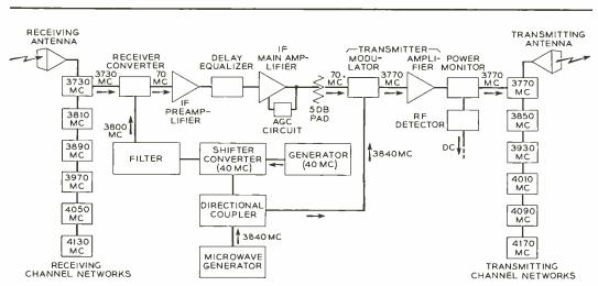
Fig. 1-Block schematic for an auxiliary repeater station.
