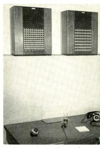
Fig. 5-A supervisor's position showing two lamp cabinets.
