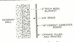
Fig. 2-Section through the side wall.
