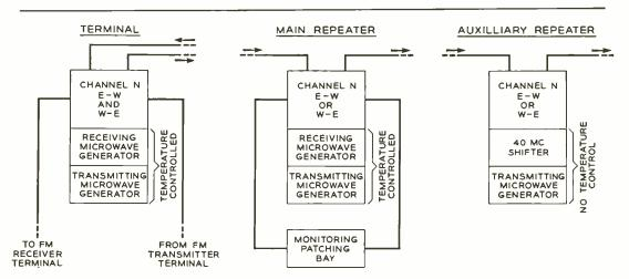
Fig. 4-Block schematic indicating the arrangement of the transmitter-receiver bay at terminal, main repeater station, and auxiliary repeater station.
