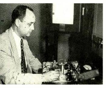
G. K. Teal measures potential gradients in npn germanium . . . hundreds of such measurements had to be made in exploring different specimens of germanium and varieties of junctions.
