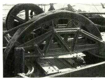
Fig. 2-The cable passing over the continuous rim of of the new dynamometer.
