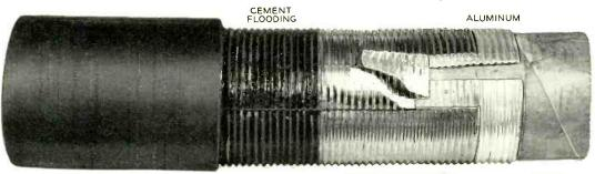
POLYETHYLENE TERNE COATED STEEL CABLE JACKET SOLDERED SEAM CORE. In Stalpeth, a layer of terne plated steel is applied over the aluminum, and the seam is soldered.
