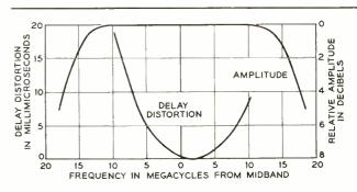
Fig. 2-Amplitude and delay characteristics of the repeater.
