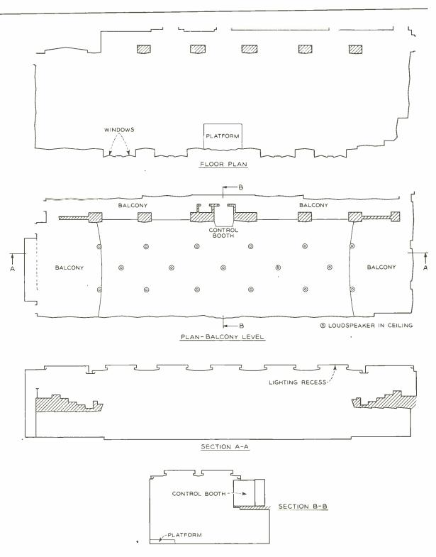
Fig. 1-Plan of Assembly Room. Angles of panels on side walls exaggerated for illustration purposes.
