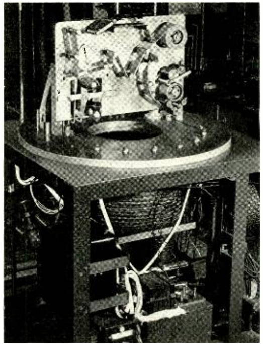
Fig. 1—Vacuum vapor-plating machine with bell jar and side panel removed. The plating occurs in the upper section normally covered with the evacuated bell jar. Below are located oil diffusion pumps, transformers, speed control and the water-cooling coils.
