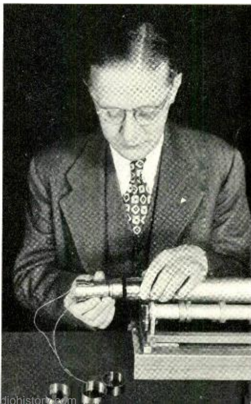
Fig. 1—H. Alfke inserting one of the accelerometers in the end of a telephone repeater.
