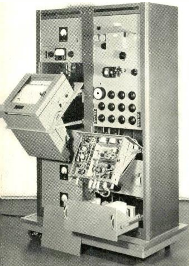
Fig. 4—Accessibility of elements facilitates servicing.
