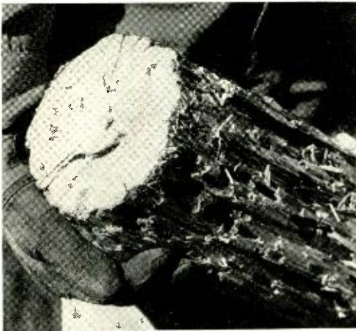
Fig. 1—Channels and galleries of dry-wood termites in the above-ground untreated section of a western red cedar pole.
