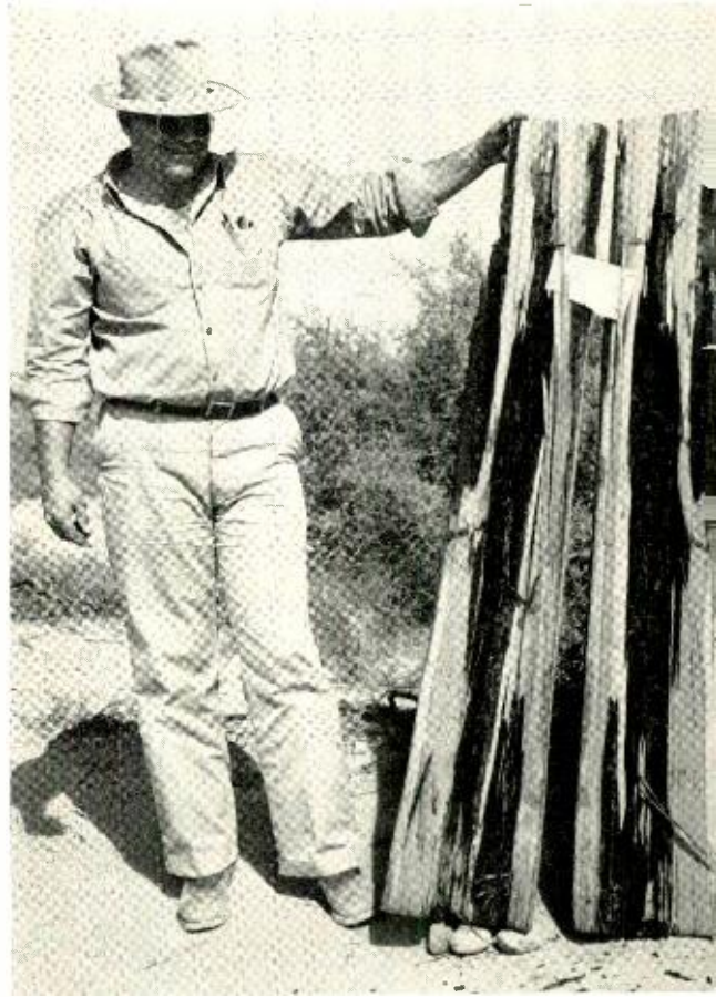
Fig. 3—R. C. C. Baker of Long Lines exhibits the dissected butt of a western cedar pole chosen as an example where an internal application of preservative eliminated a colony of dampwood termites.
