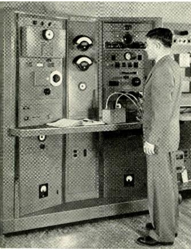
Fig. 6—Operating the phase and transmission measuring set designed for video frequencies.
