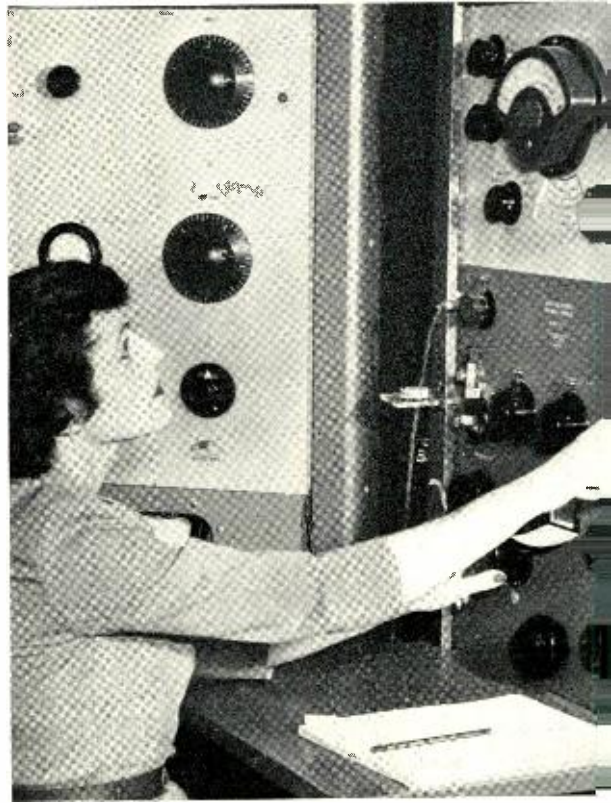
Fig. 4, at right—Using a high frequency Maxwell bridge, the operator checks inductance of the toroidal specimen on the shelf, right of center.
