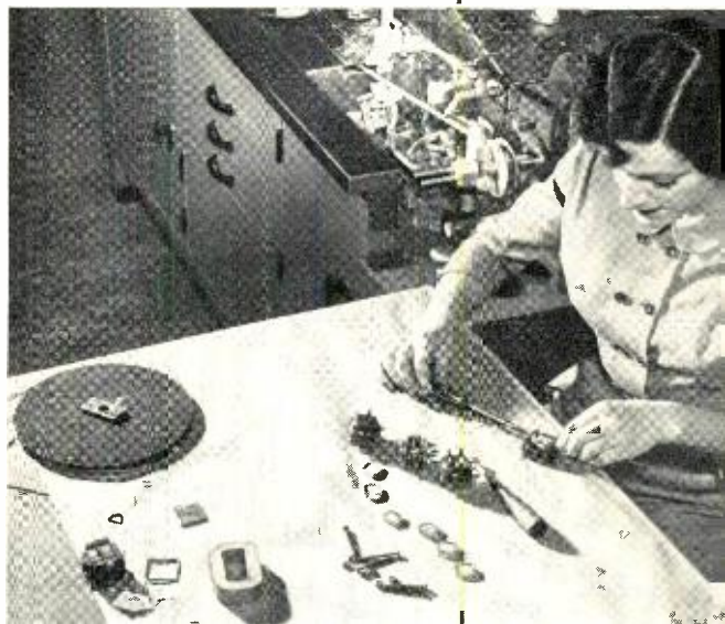
Fig. 2—Adele Aboutok clamps rectangular cores prior to their heat treatment. The cataphoresis insulating machine is in the background.
