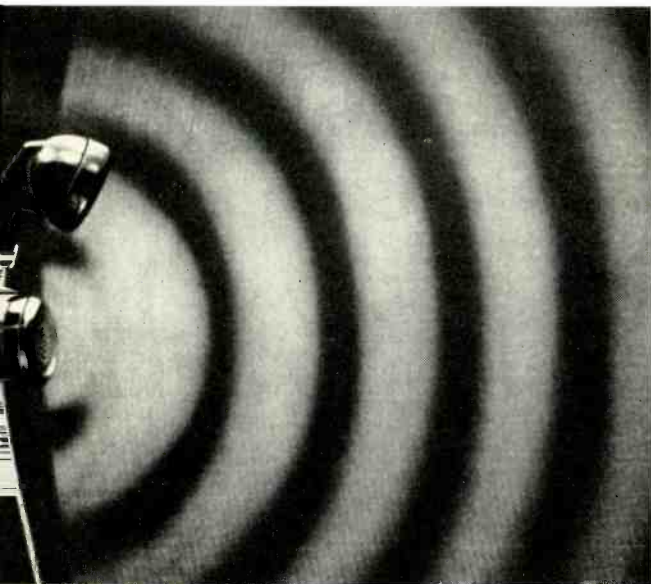
Pattern of sound waves from a telephone handset.
